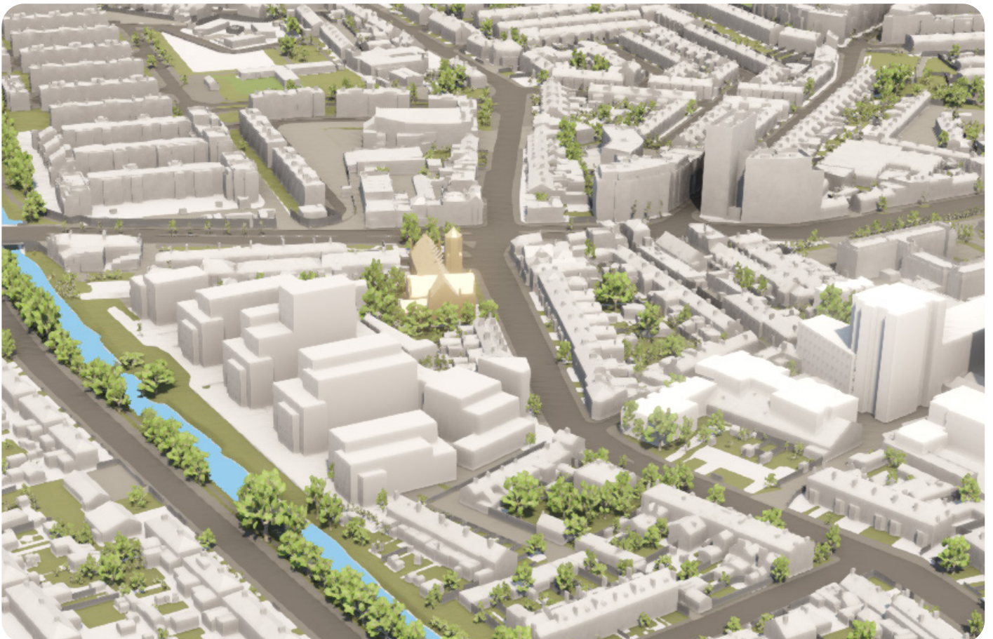
Figure 30: Proposed development on the Example Site in context showing the reduction in scale of the proposal at the edges of where prevailing heights are lower and the intensification of development in the less sensitive centre of the site
